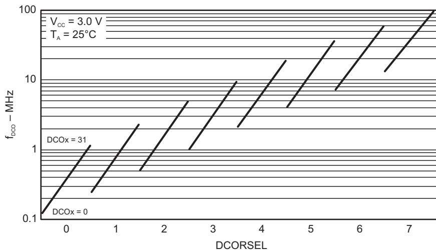
Figure 5-11. Typical DCO Frequency
